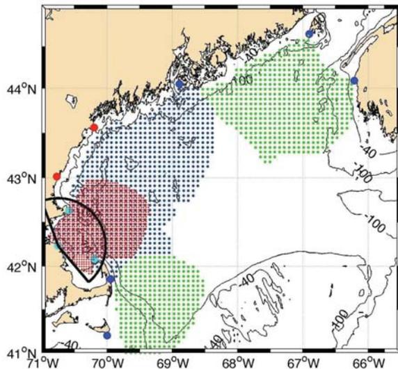
**B) High Frequency Radar (HFR) locations.** Existing (green) and proposed additional (blue) coarse resolution HF radar coverage along with proposed high resolution (red) coverage of the western GoM and Mass. Bay. Locations for all GoM sites are shown in (blue) for present-day sites, (red) near-term expansion using equipment on loan from Rutgers, and (cyan) higher frequency sites. The ideal coverage area for the standard range site proposed here is shown in black.
